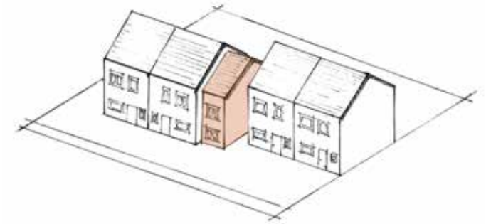
Double storey side extension
